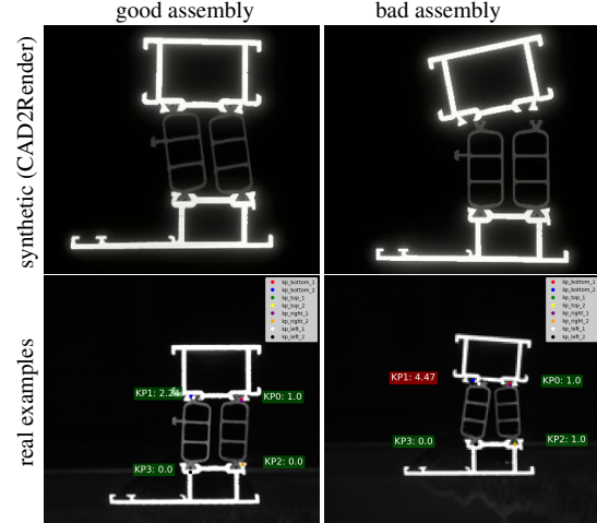
Figure 10. Assembly validation of good and bad assemblies. Top: synthetic examples generated with CAD2Render. Bottom: Output of the model shown on top of real examples in the case of a good validation (all points within spec) and a bad validation (one of the insertion areas show points that are too far from each other).
