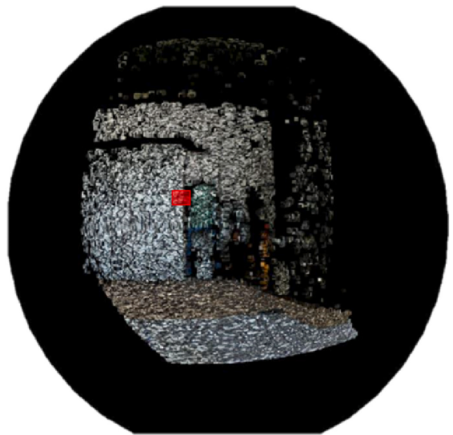
Fig. 12. The front view of the four-pi Compton camera image is superimposed with the point cloud. A mask is applied to display only the top 1% of the highest radiological values, and the hotspot location is highlighted in red. (For interpretation of the references to color in this figure legend, the reader is referred to the Web version of this article.)
