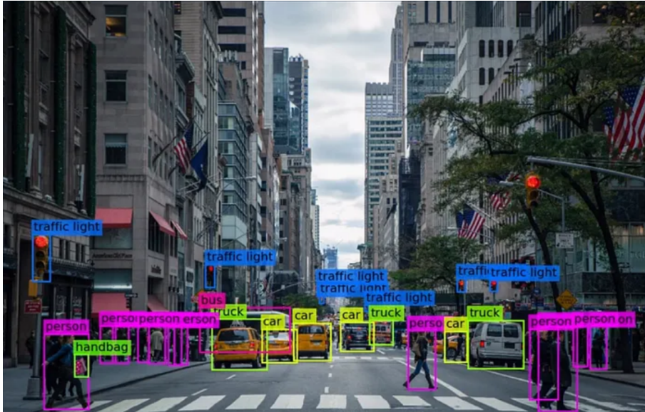
Figure 3.1: Example of YOLO’s output detecting several basic objects
