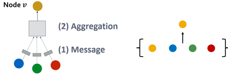
Figure 4.5: Aggregate and combine the feature vector of node v [Les23].
