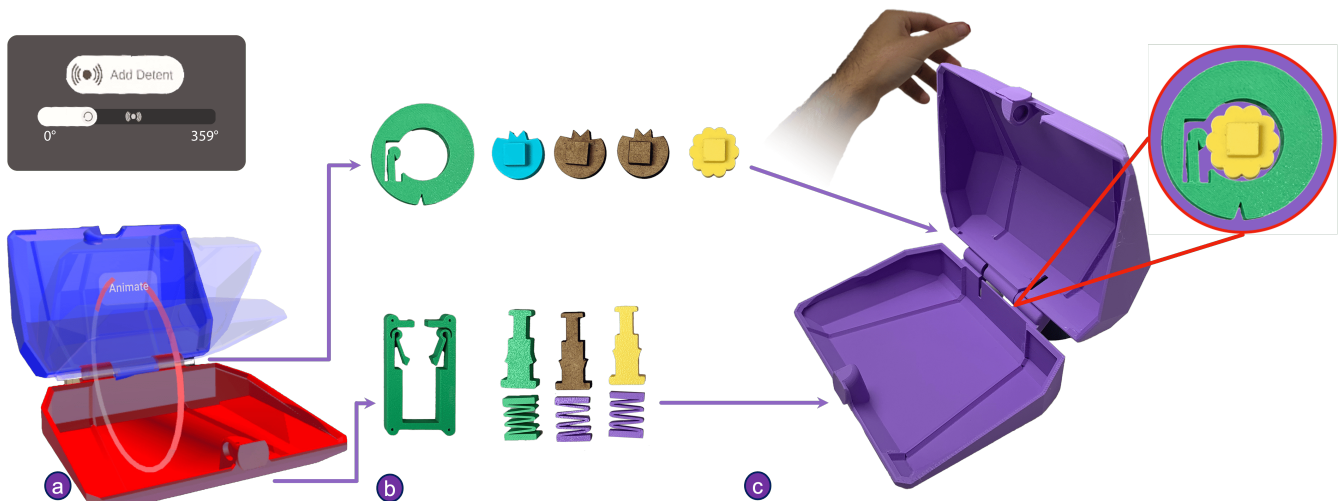
Figure 1: A future workflow for designing the haptic feel of a moving part. (a) The tool in which the designer chooses the motion type (e.g., sliding or rotating) and describes how it should feel, such as clicks or resistance. (b) The system fabricates several swappable internal pieces that can be placed into the 3D-printed object, each creating a different feel. (c) The designer installs the pieces one by one and tries the object to decide which feels best.
