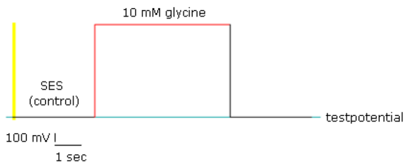
Figure 4. Protocol for the current-voltage relationship. The control and 10 mM glycine test condition are applied in the same trace. The test potential increased with 20 mV after every trace, starting at -100 mV up to +80 mV.
