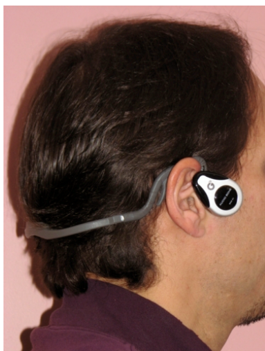
Figuur 2.6: Bone-conducting headset: Audiobone van Goldendance Co., Ltd. (Lindeman et al. 2008)
