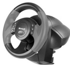
Figuur 4. 1 DOF: Microsoft® SideWinder Force Feedback Wheel
