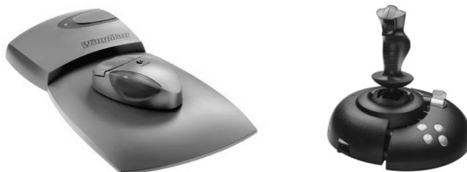
Figuur 5. 2 DOF: (links) Logitech® WingMan Force Feedback Mouse (rechts) Microsoft® SideWinder Force Feedback joystick
