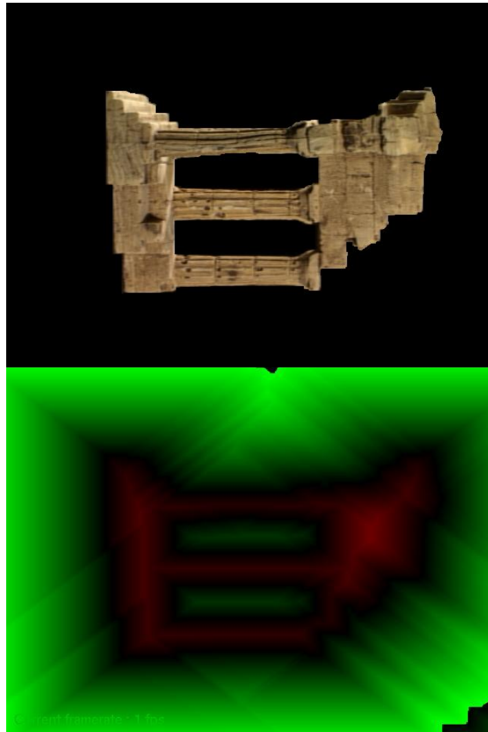
Figure 3.8: The result after the preprocessing stage. Red pixels indicate how far inside the silhouette while green pixels indicate how far outside the silhouette
