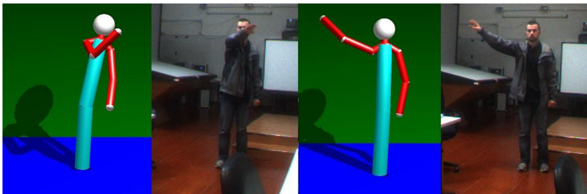
Figure 3.19: After locating the hands and the face of the player the pose is estimated using the Jacobian transpose method.
