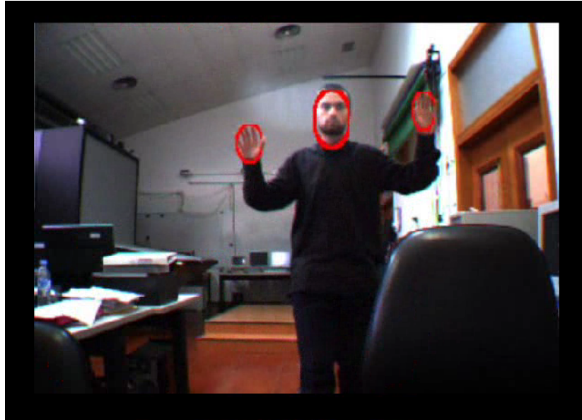
Figure 3.16: Face and hands detection algorithm
