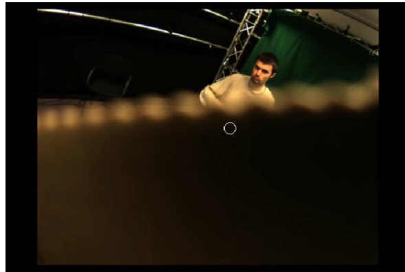
Figure 4.3: The projection of the red ball is invisible on this camera, but because it is visible at two other cameras the location can still be calculated [27].
