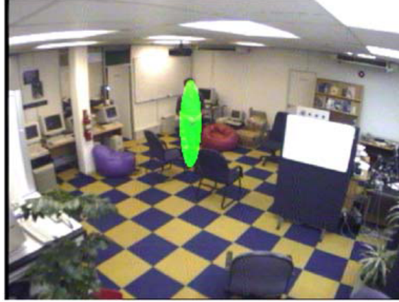
Figure 2.16: The result of tracking a person using the extended Kalman filter. An ellipsoid is drawn on the location of the person [17].
