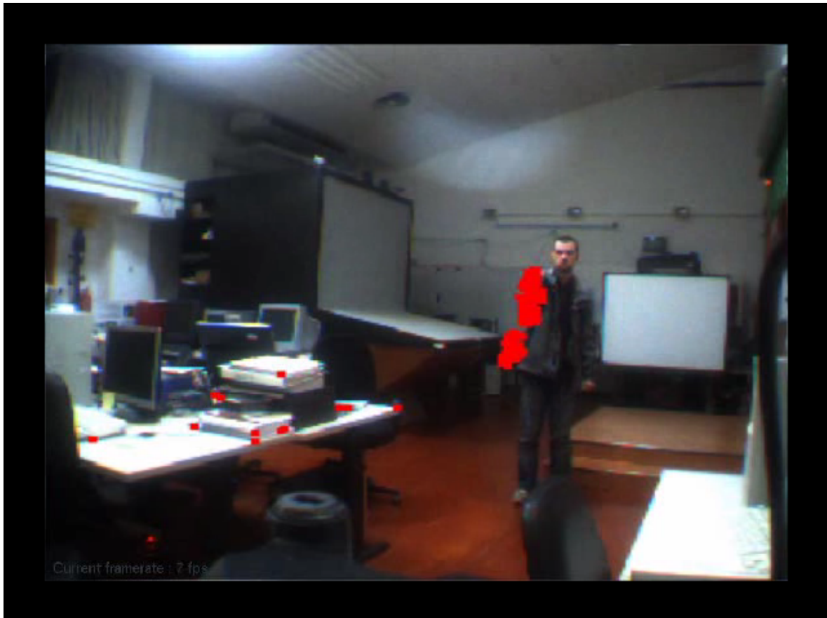
Figure 4.4: A 3D drawing game which records motion and use the depthmap to define the location of the motion in space. When the player moves further than a predefined distance from the camera, the motion is ignored. When he puts his hand in front of him, the motion is closer to the camera and the pixels are colored red. The red dots on the leftside of the image are created because of noise.
