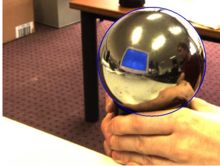
Figure 4.16: Locating the spherical mirror: robust ellipse detection.
