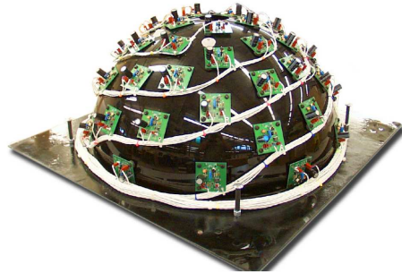
(b) Polynomial Texture Map setup of Malzbender et al. [Malzbender 01].
