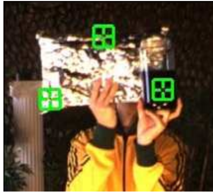
Figure 3.28: We can track markers behind highly specular surfaces and behind materials that are opaque for visible light but transparent for infrared light such as coke.
