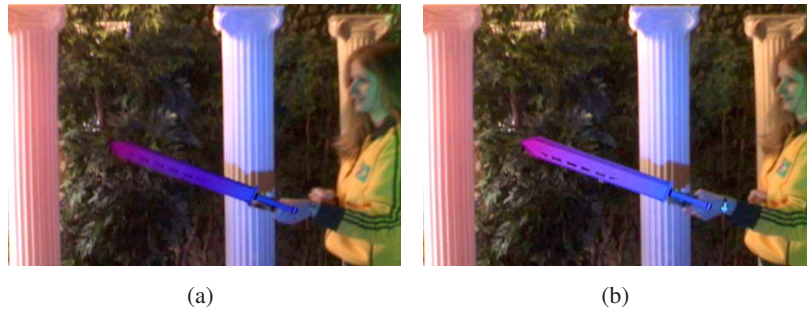
Figure 3.26: A stick, with markers attached to it, is rotated. Our system is able to track this movement as is shown by rendering a virtual sword in place of the tracked stick. Motion tracking systems that calculate the orientation of surfaces from position information have problems to track this kind of motion of thin objects, because there is not enough space to place the required markers.
