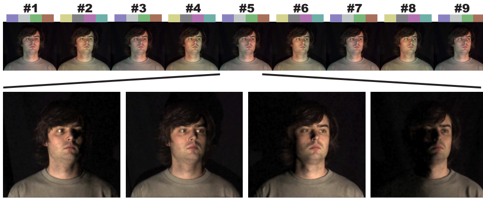
Figure 4.1: Demultiplexing illumination using our method. Top row: 9 input frames of a dynamic scene. A person is lit by only 2 different colored illumination patterns using 4 differently colored light sources (indicated by the squares). Bottom row: The output images show the demultiplexed lighting. I.e., each image contains the result of having illuminated the scene by each source separately.
