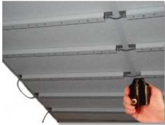
Figure 3.2: Using the HiBall system [Welch 97], a marker which contains multiple light sensors senses the amount of light arriving from a number of LEDs attached to the ceiling to calculate its position.
