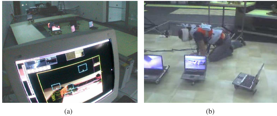
Figure 3.5: Laptops attached to robots are tracked by our system to create peephole displays during a theatre play.
