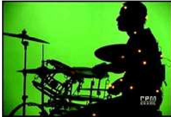
Figure 3.1: In the PhaseSpace system [inc 07], a number of LEDs are attached to points of interest. These points are tracked using multiple high speed cameras to obtain their 3D position.
