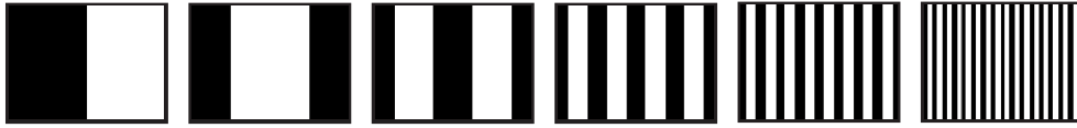
Figure 4.4: When these patterns are projected onto a scene one after the other, each point in the scene is labeled with a unique code that corresponds to a given column in the projector. This can be used to establish camera-projector correspondences.
