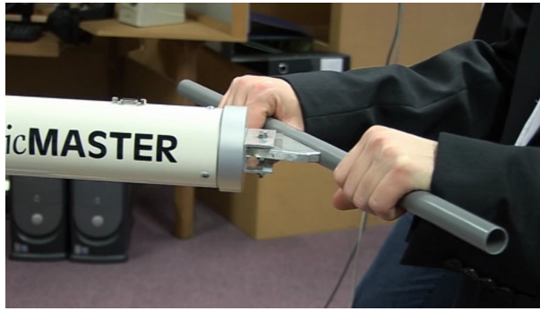
Figure 5: The Hapticmaster with shopping cart handle used for navigation.
