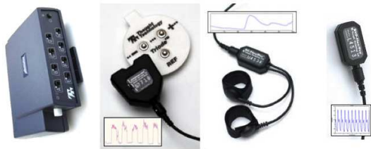
Figure 2: ProComp Infniti encoder and the physiological sensors: EMG, GSR, BVP (from left to right).
