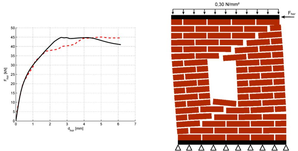
Figure 3: Load-displacement curve and deformed mesh for the shear wall test
