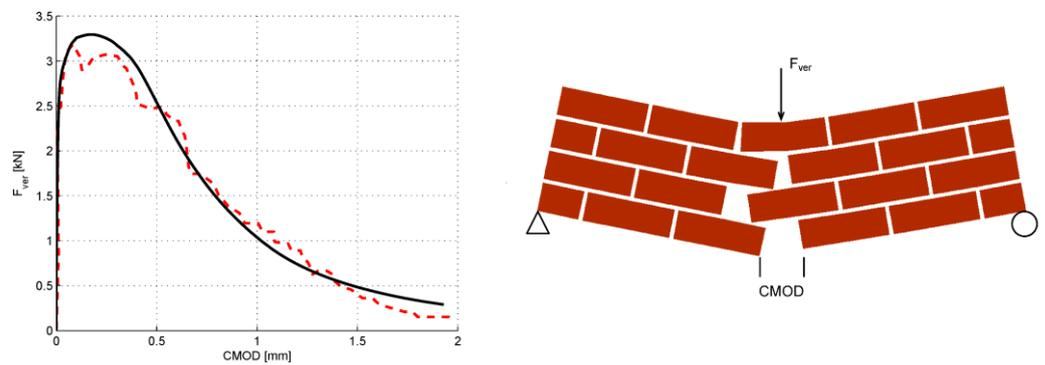
Figure 2: Load-CMOD curve and deformed mesh for the three-point bending test
