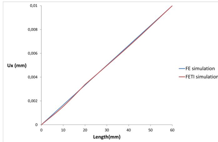
Figure 6: Displacement field at height 10 mm
