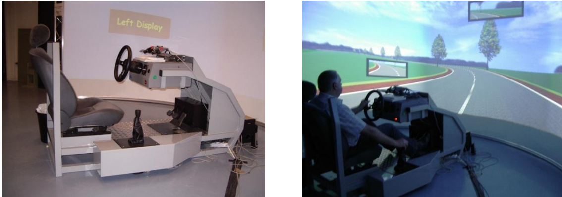
Figure 21 IMOB-driving simulator on the basis of the STISIM Drive™-technology
