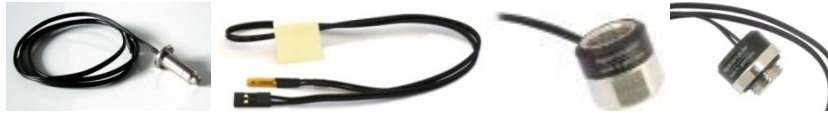
Figure 5 : NTC thermistor types used in experimental heat extraction set-up. Far right; NTC thermistor build in metal shielding. Right; 'Naked' NTC thermistor. Far Left; NTC thermistor build in piece of metal tubing, screw thread on the outside. Left; same type as upper left but with screw thread on the inside. All sensor measure between 1 and 2 cm.
