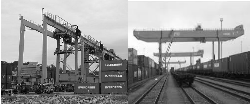
Figuur 5: Rubber tyred gantry crane en rail mounted gantry crane (Bron: Wikipedia).
