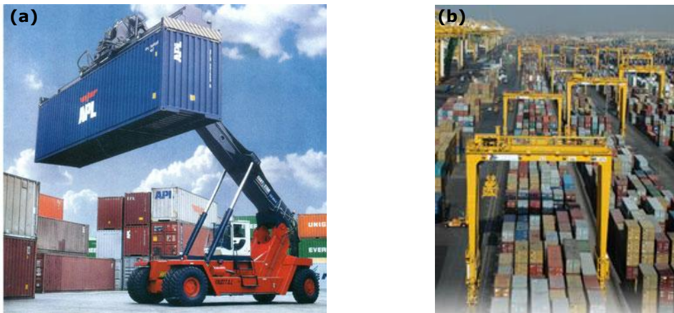
Figuur 16: (a) Reach stacker (Ronak Container & Cargo Logistics Pvt. Ltd., 2010) en (b) Yard kraan (Bromma, z.d.)
