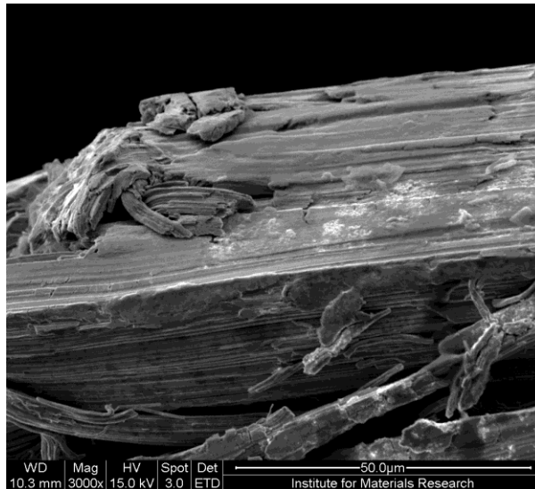
Figure 20: SEM image of tip NCD coated Ir wire (L11020D)
