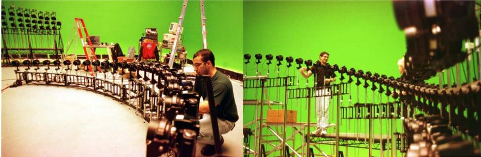
Figure 1.3: Camera setup used in the *Matrix Trilogy*, used to create the “bullet time” rotating camera effects. (<http://whatisthematrix.warnerbros.com/>)
