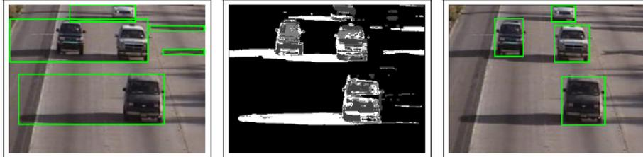
Figure 2.2: **Importance of shadow handling in traffic surveillance.** [Prati 01]
