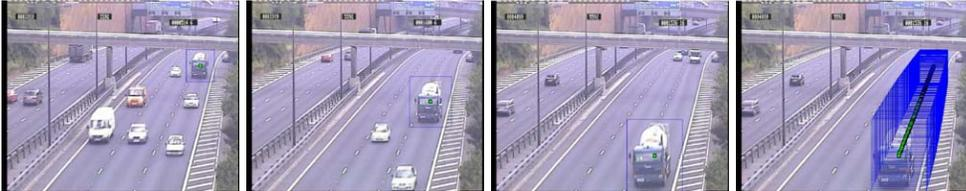
Figure 2.8: **Vehicle trajectory calculation.** Windows drawn around a particular vehicle by the user, with on the right a calculated trajectory for the vehicle.
