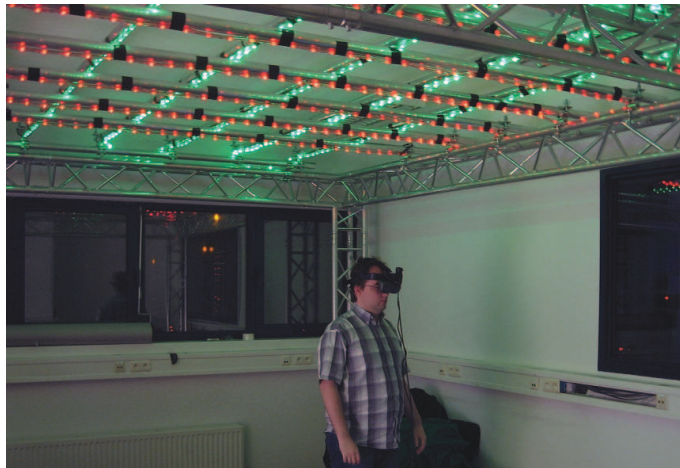
Figure 1: Our lab set-up with a 4 by 3 meter grid of LED ropes on the ceiling. The camera mounted on the virtual reality glasses tracks its position and orientation by filming this grid.
