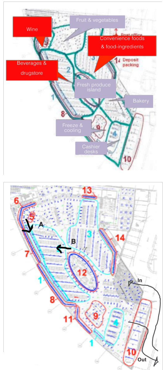
Figure 5.23. Floor plan of Plus: The red tags are the zones that contained dynamic lighting. Zones 1, 2 and 3 with dynamic fluorescent tubes and zones 6, 7 and 8 with the coloured LEDs. Source: Philips
