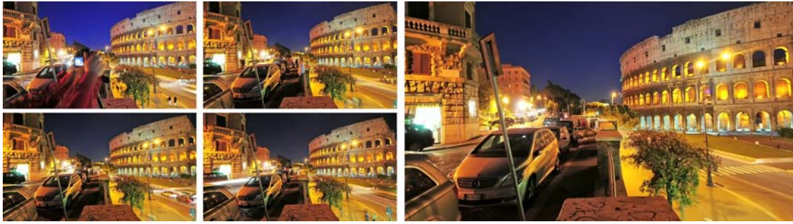
Figure 3: Result from a video input using 40 frames. The camera, the cars and the tourists before the Colosseum are successfully filtered out. There is a difference in lighting in the different input images, but this is not noticeable in the final result.
