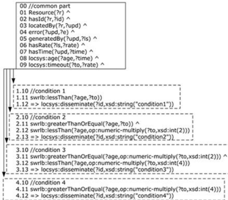
Listing 5.1. A combined representation of the SWRL rules that use the localisation ontology to infer about a corresponding resource's appropriate visualisation condition based on this resource's location tracking status.
