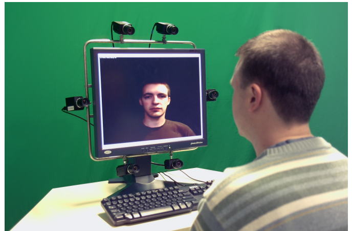
Fig. 1. Example setup of our immersive one-to-one teleconferencing system, using multiple cameras to allow virtual camera image generation.
