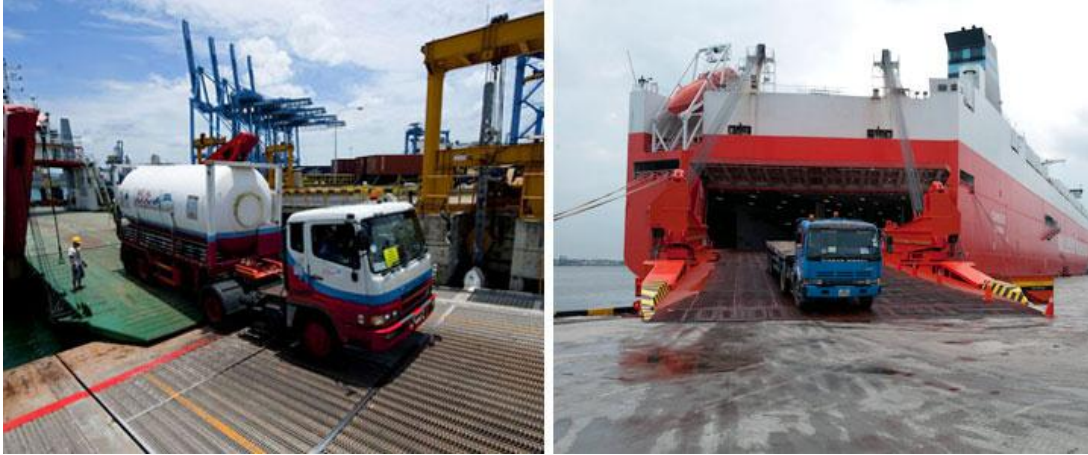
Figuur 11 - Roll on/Roll off principe (Jurong Port, Roll on, Roll off (Ro-Ro) Facilities, internet, 02-02-2012, http://www.jp.com.sg/JurongPort/roll-on-roll-off-ro-ro-facilities )
