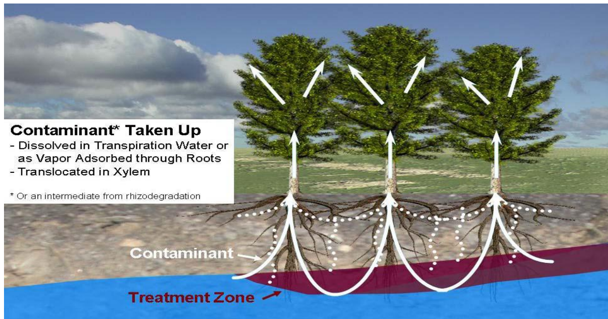
Figuur 8: Fyto-extractie principe. Bron: (The Interstate Technology & Regulatory Council Phytotechnologies Team 2009).
