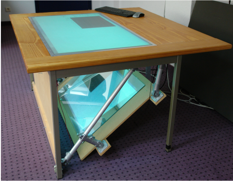
Figure 3.2: The custom-built FTIR tabletop used during the evaluation provides a 50-inch touch-sensitive surface, with a resolution of 1920 by 1080 pixels.
