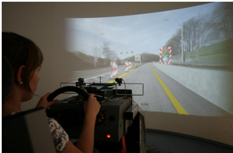
FIGURE 3 Traffic Sign Simulator mock-up with eye-tracking system.
