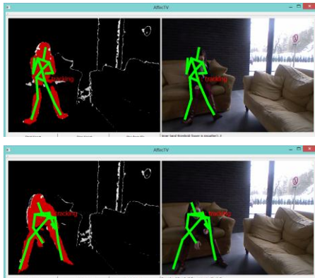
Figure 3 Screenshots of posture capturing software optimized for sitting postures using depth camera.
