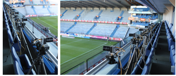
Figure 2: Overview of the camera setup. The setup consists of 8 computer vision cameras with 25mm lenses placed 1 meter apart from each other.
