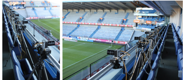
Fig. 2. Example of the camera line setup. Cameras are placed approximately one meter apart from each other. The distance to the field is about 20 meters.
