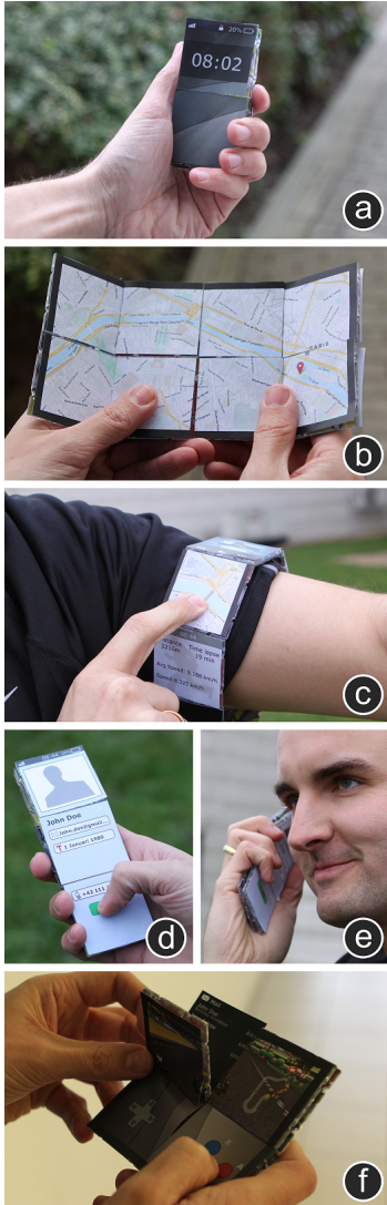
Figure 4: The 2x4 Rubik's Magic folding plate puzzle enables various form factors for mobile devices.
