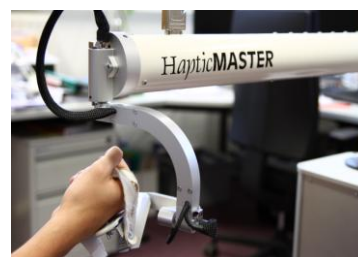
Figure 2. I-TRAVLE hardware system: MOOG HapticMaster and visual display (top), ADL Gimbal (bottom)
