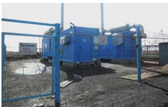
Fig. 46. Methane capture installation on the surface of the ArcelorMittal coal mine in Karagandy.
