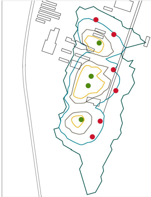
Figure 3.28 Location of the extraction wells at the source zone and the borders of the site
