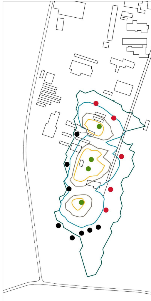
Figure 3.26 Location of the extraction wells for the P&T system (green dots), bioremediation cells (red dots), and recharge wells (black dots)
