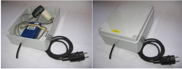
FIGURE A22: Aethalometer model AE51 (AethLabs, 2011) in a weatherproof housing. On most measurement sites an extra battery was placed inside the housing, so no other external power was necessary.
