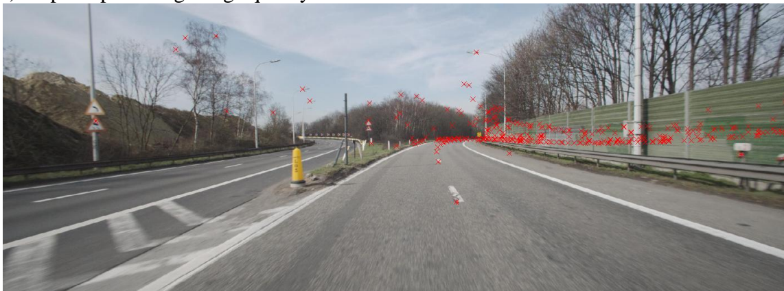
b) Step 2: camera-tracking of 3D reference points
