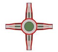
Figure 3a – Roundabout with separate cycle paths – priority to bicyclists
