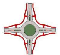
Figure 4 - - Roundabout with grade-separated cycle paths
