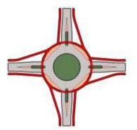
Figure 3b – Roundabout with separate cycle paths – no priority to bicyclists
