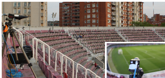
Figure 2: The camera setup. 7 cameras are visible, set up in an arc arrangement. The distance is 10 meters between the cameras.
