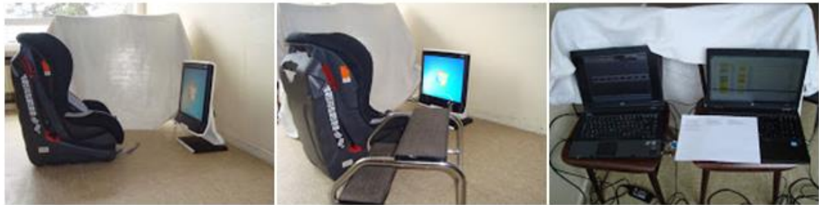
Figure 2 Test environment at daycare center 'De Ukkies': Tobii T120 monitor and car seat (left), Tobii T120 monitor, car seat and little seat for the accompanying caregiver (middle), and hidden computers for data registration (right).
