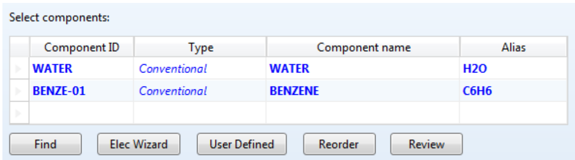
Figure 11: Adding components for a liquid-liquid system in Aspen Plus.
