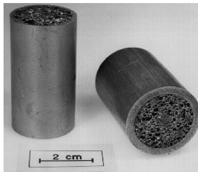
Figuur 15: Aluminiumschuim in aluminium buisprofiel [22]
