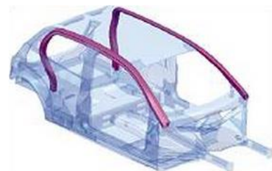
Figuur 6: tailored tubes in autoframe [10]
