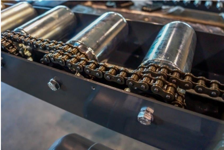
Fig. 13 Rollenbaan kettingaandrijving (Borst_systems, 2014)
