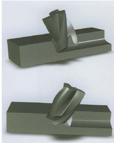
Figure 5-8: Upper example shows a lead cut, lower example shows a lag cut (Arpo, 2008)
