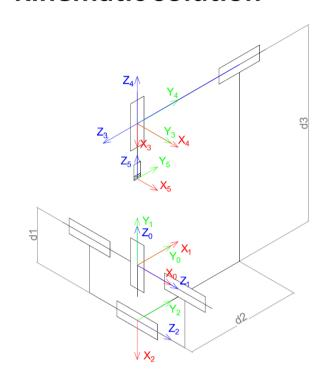
Denavit-Hartenberg method to convert coordinates between frames. This results in a machine specific transformation matrix.
