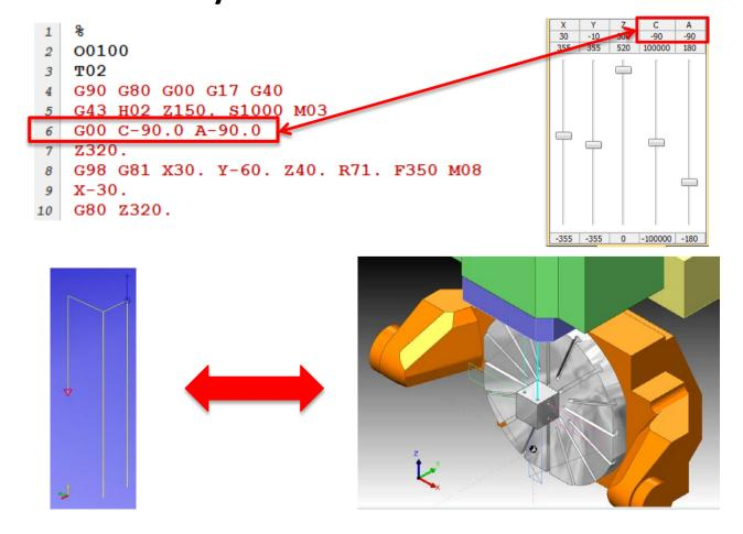
On the left the resulting G-code is shown with below its toolpath. On the right the CAM simulation with the machine values are shown. From this analysis we can conlcude that the transformation matrices are correct and the G-code is excecuted in the correct order.
