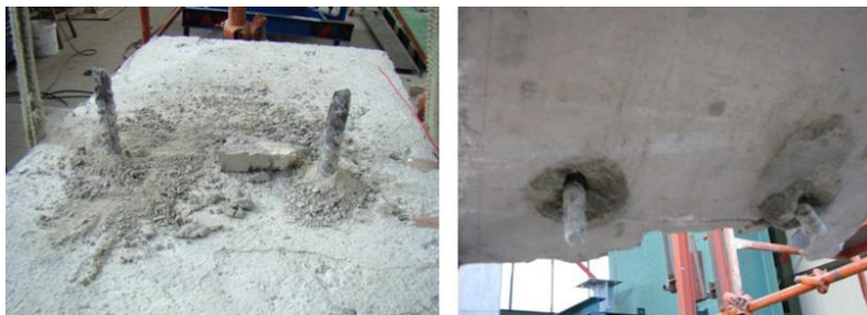
Figuur 2.22: Stalen verbinding faalt [17]
