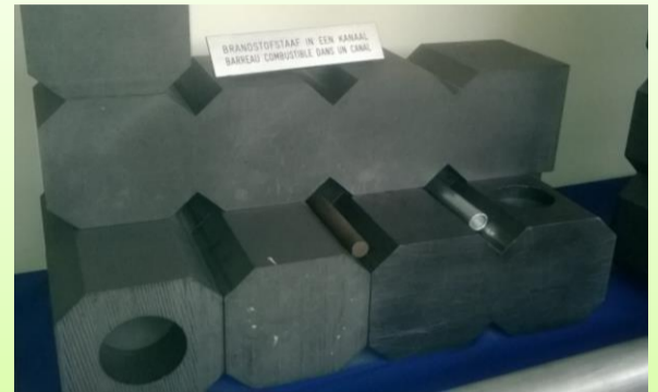
Figure 1: Spare blocks of BR1 graphite moderator
